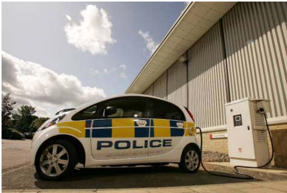
Mitsubishi iMIEV connected to a TEPCO Rapid charge station
